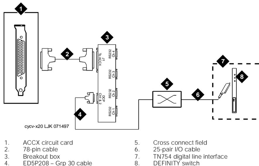
**Figure E-8. Connecting Lucent INTUITY to the Network Through Two DCP Lines**
