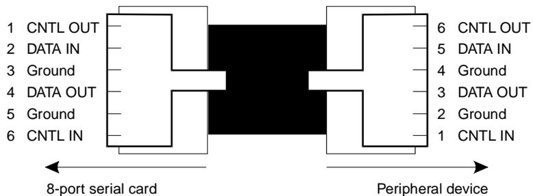
**Figure D-2. Pinout Connections for Modular Jacks on the Multi-port Serial Circuit Card**
