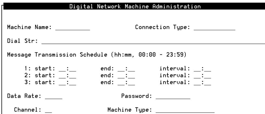
**Figure 13-5. Digital Network Machine Administration Window**
