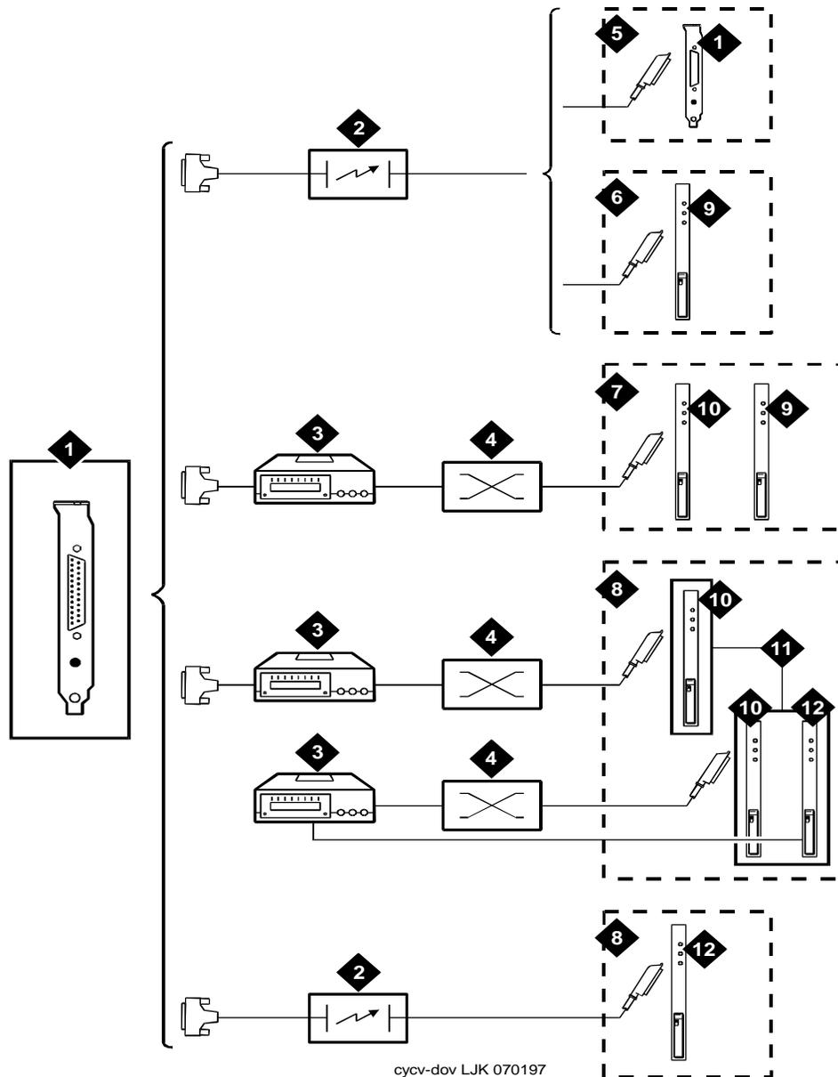
Figure E-1. Overview of Platform Switch Cable Connections
