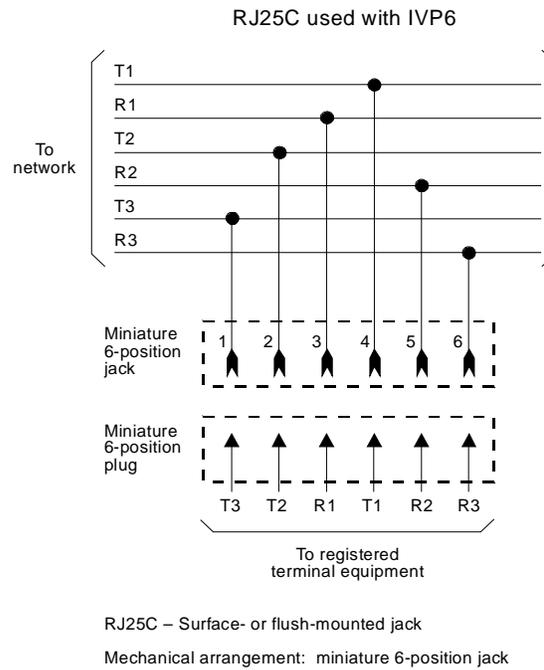
**Figure D-1. Wiring and Pin Diagram for the IVC6 Tip/Ring Circuit Card**
