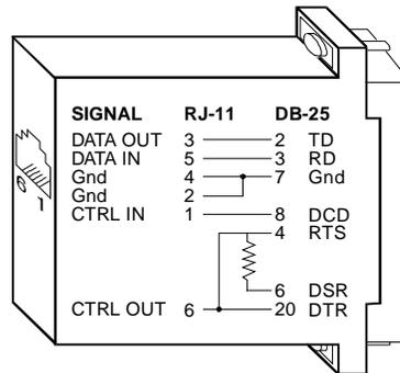
**Figure D-3. Pinout Connections for DTE or DCE Devices**
