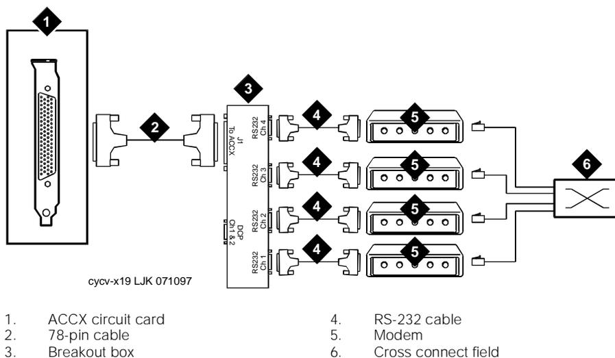
**Figure E-10. Connecting Lucent INTUITY to the Network Through Four RS-232 Cables**
