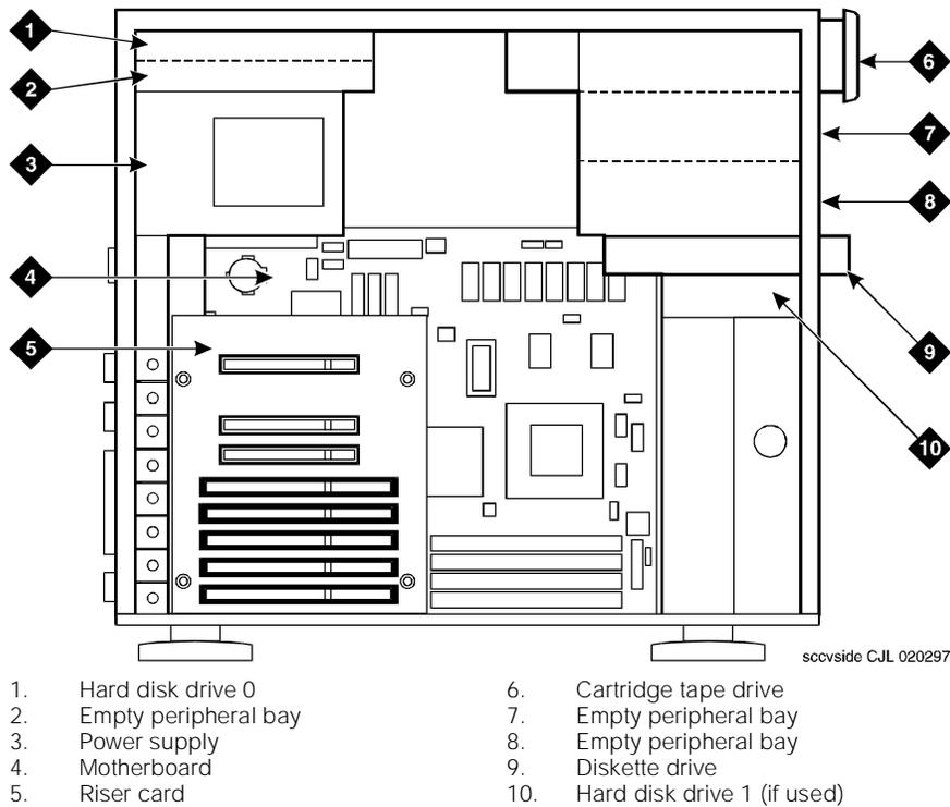
**Figure 2-7. Side View of MAP/5P Including Locations of Peripheral Drive Devices**
